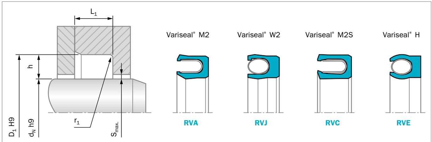
Figure 18: Installation drawing
