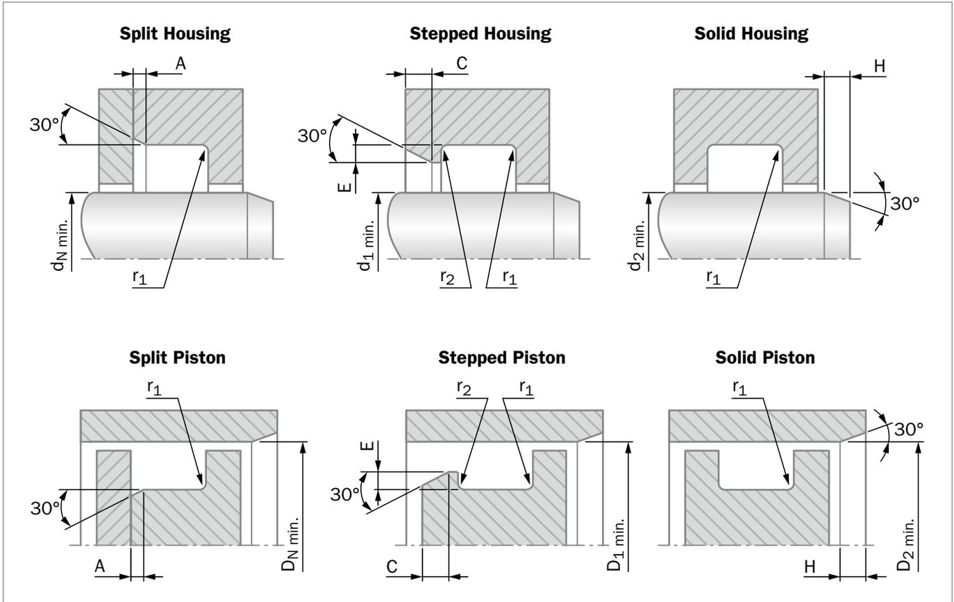
Figure 11: Variseal® groove configurations
