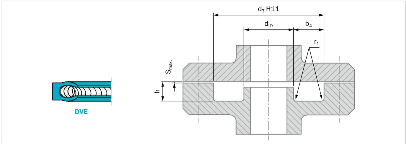
Figure 26: Installation drawing
