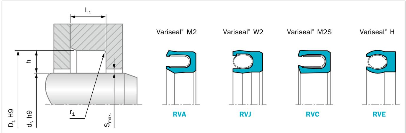
Figure 19: Installation drawing
