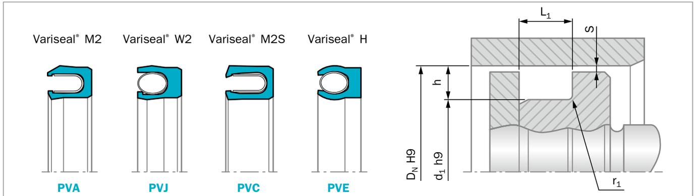
Figure 22: Installation drawing
