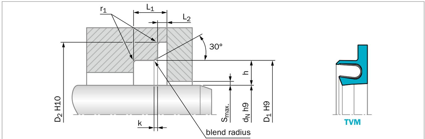
Figure 32: Installation drawing
