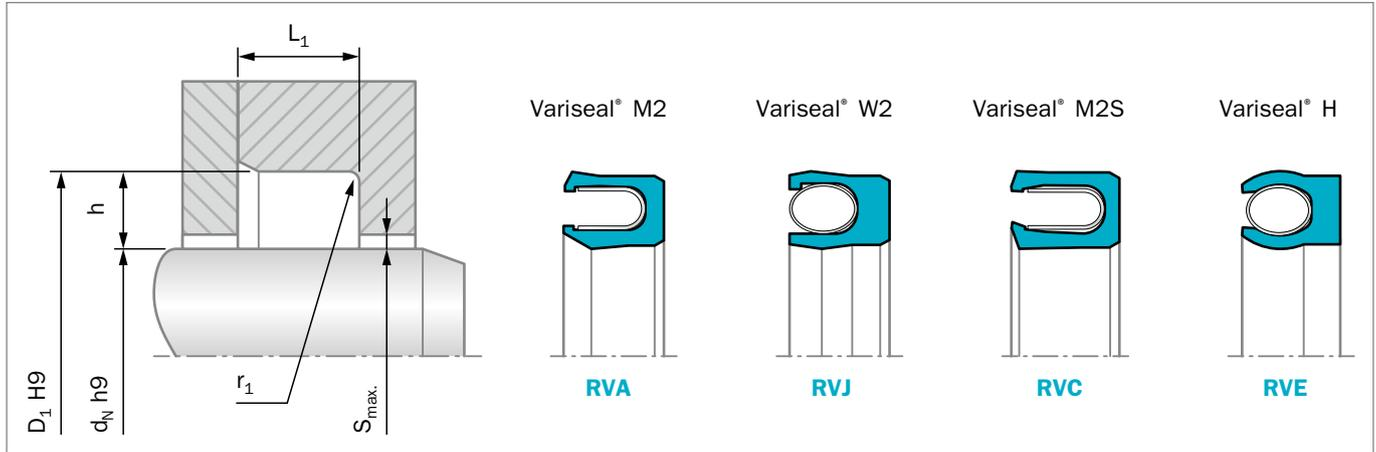
Figure 20: Installation drawing
