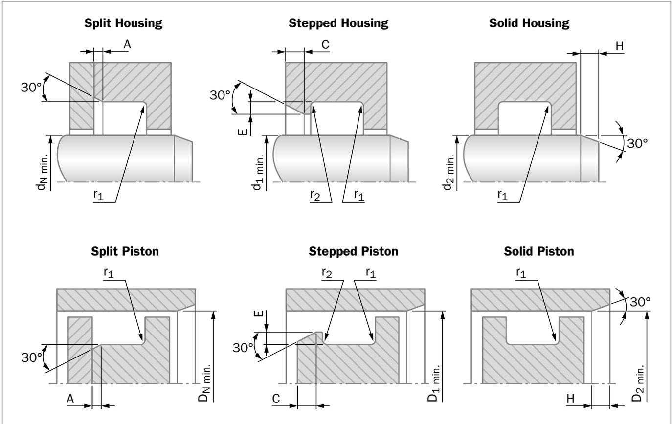
Figure 10: Variseal® groove configurations
