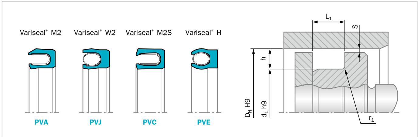
Figure 23: Installation drawing
