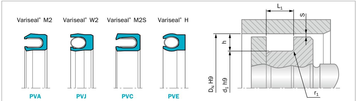
Figure 21: Installation drawing
