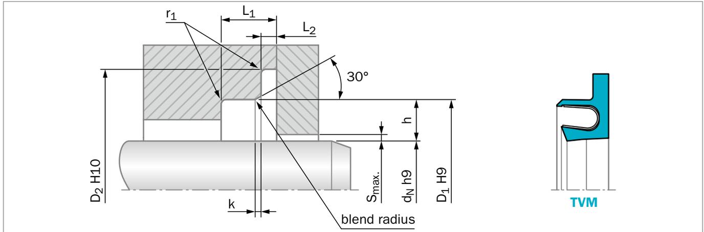
Figure 31: Installation drawing
