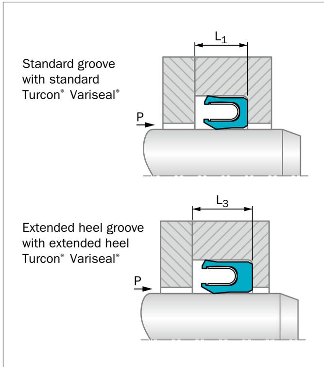
Figure 35: Standard Turcon® Variseal® and Turcon® Variseal® with extended heel
