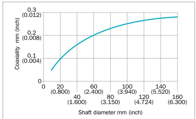
Figure 12: Coaxial tolerance capability
