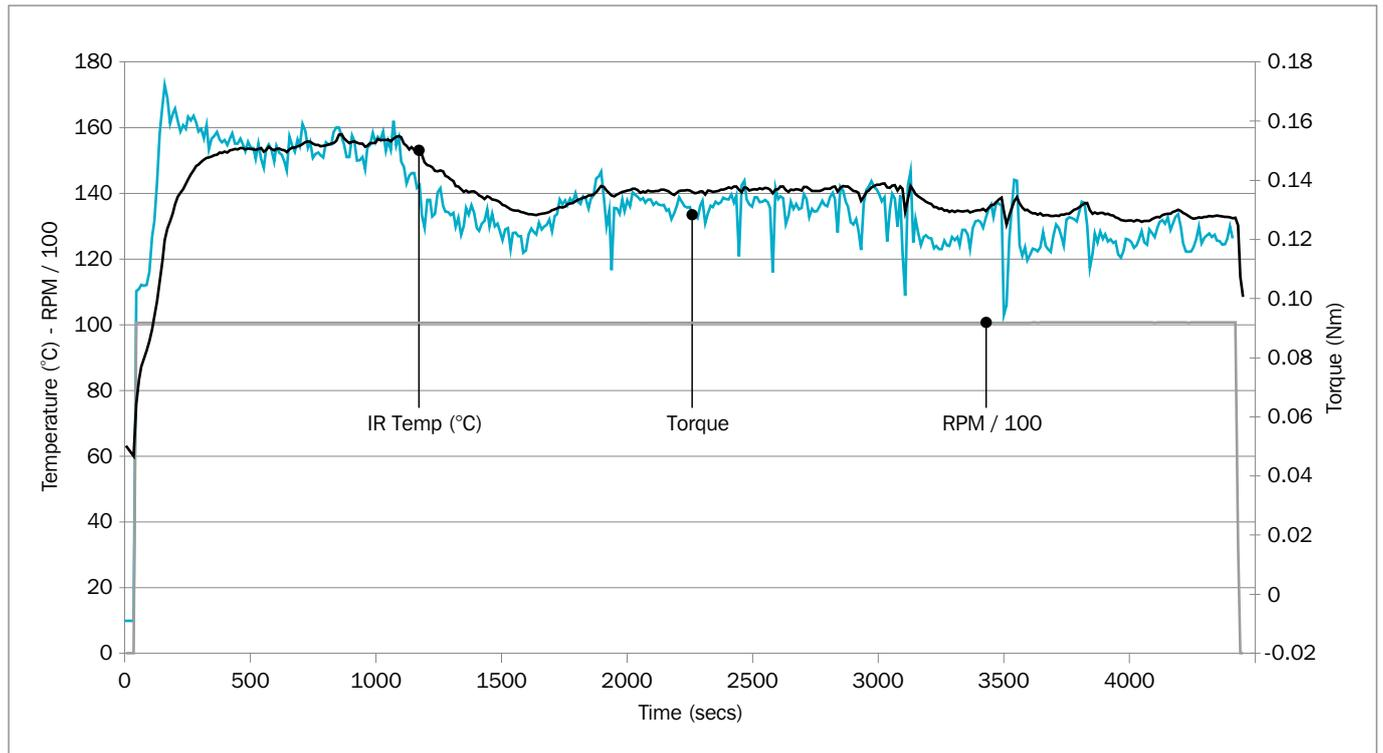
Figure 10: Running torque for Turcon® Varilip® PDR
