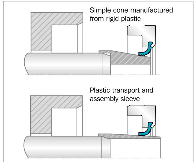
Figure 16: Assembly tooling types for installation on shafts
