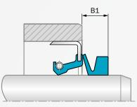
By installing Forsheda® V-Ring as shown, adequate protection is granted to the Radial Oil Seal and system service life is increased.
