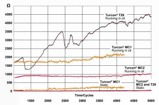
Turcon<sup>®</sup> MC1 Medium-filled material for dynamic applications requiring medium to high conductivity Turcon® MC2 High-filled material for dynamic applications requiring high conductivity
