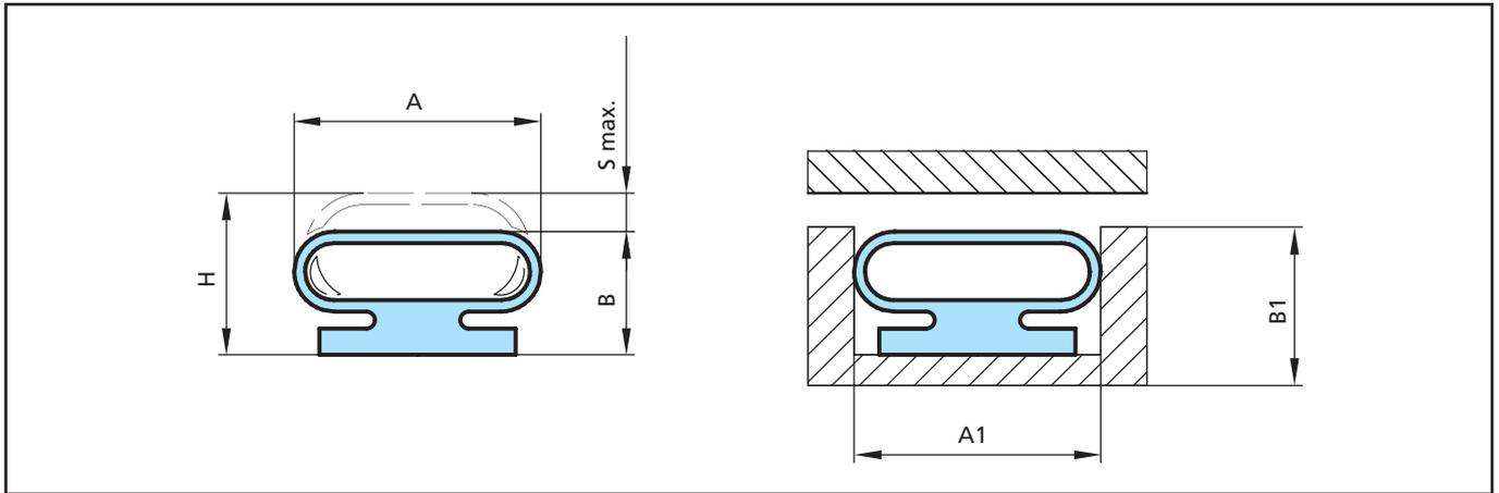
Figure 17 Low-Pressure – with smooth wide sealing surface
