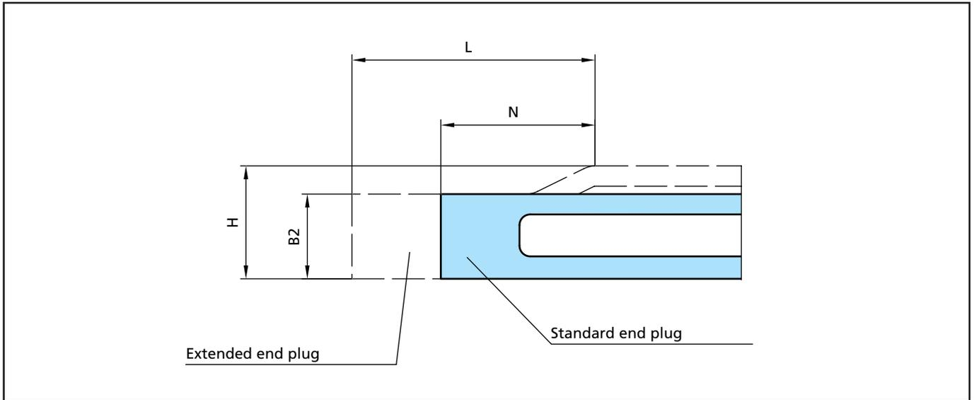
Figure 38 End plugs for high-pressure profile
