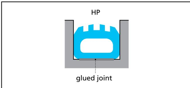
Figure 5 Installed high-pressure Airseal in groove
