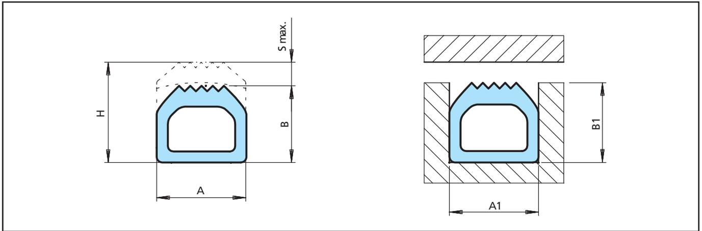
Figure 27 High-Pressure – with peaked sealing profile
