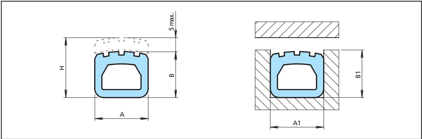
Figure 24 High-Pressure – with smooth sealing profile and grooves
