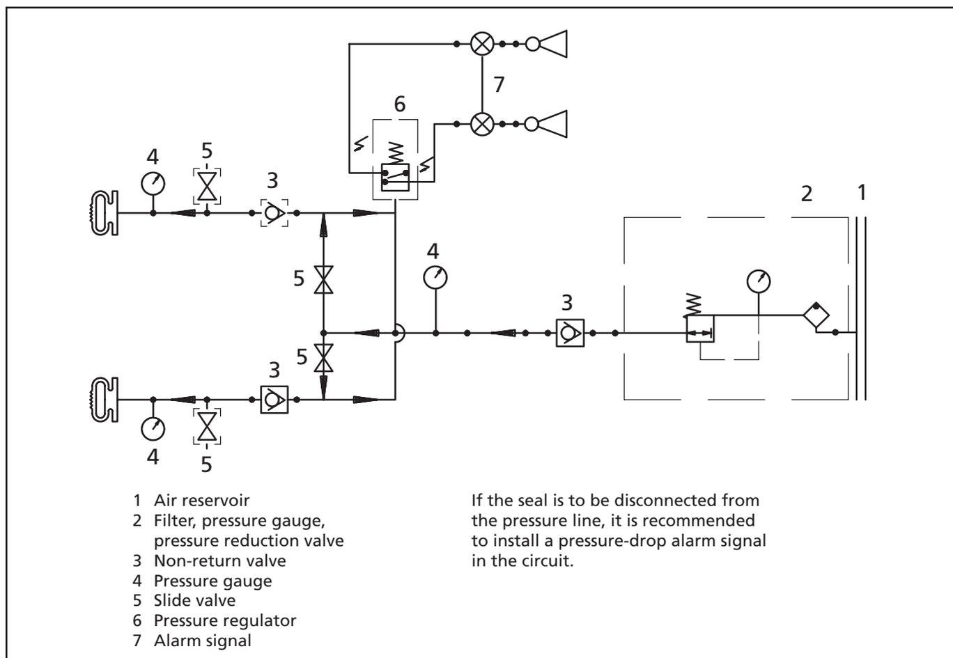
Figure 7 Circuit diagram – Airseal
