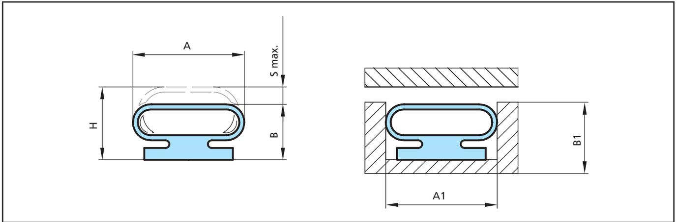
Figure 15 Low-Pressure - with smooth wide sealing surface
