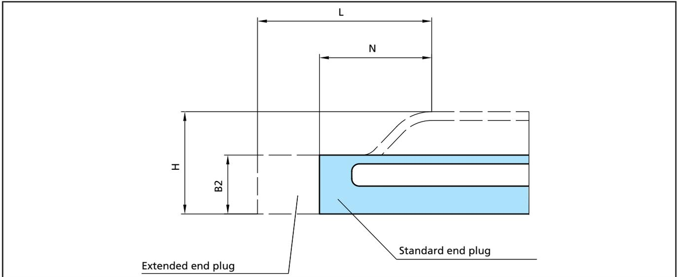
Figure 40 End plugs for low-pressure profile
