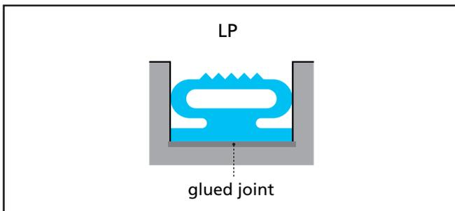
Figure 6 Installed low-pressure Airseal in groove
