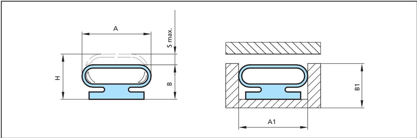
Figure 14 Low-Pressure - with smooth wide sealing surface
