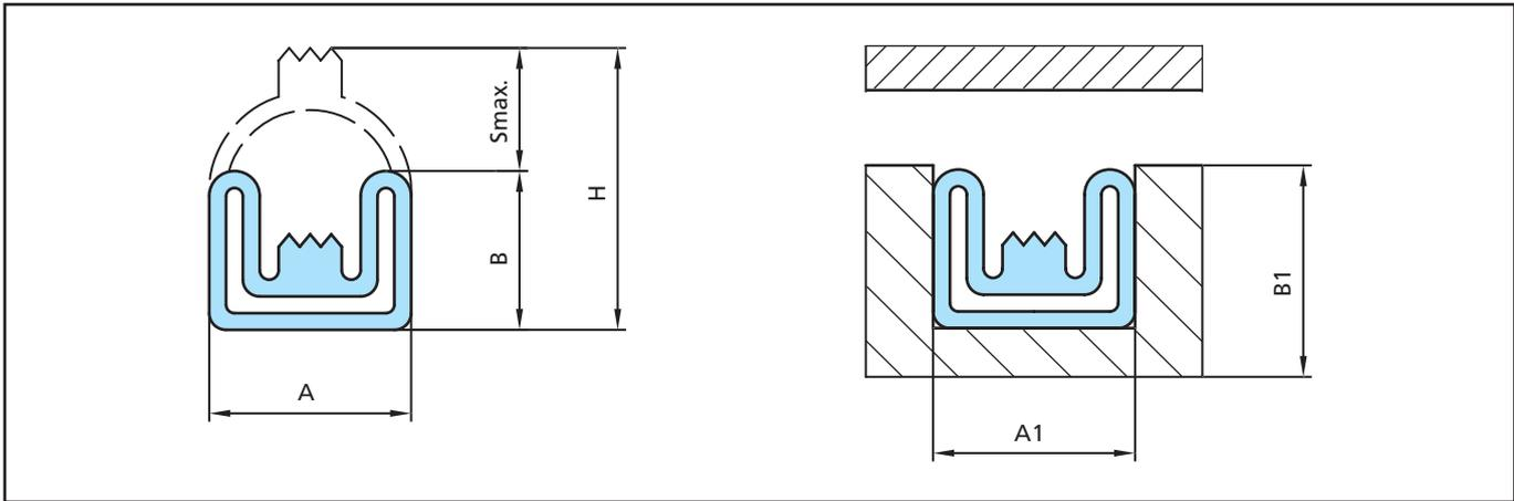
Figure 22 Low-Pressure – with specially formed sealing edge
