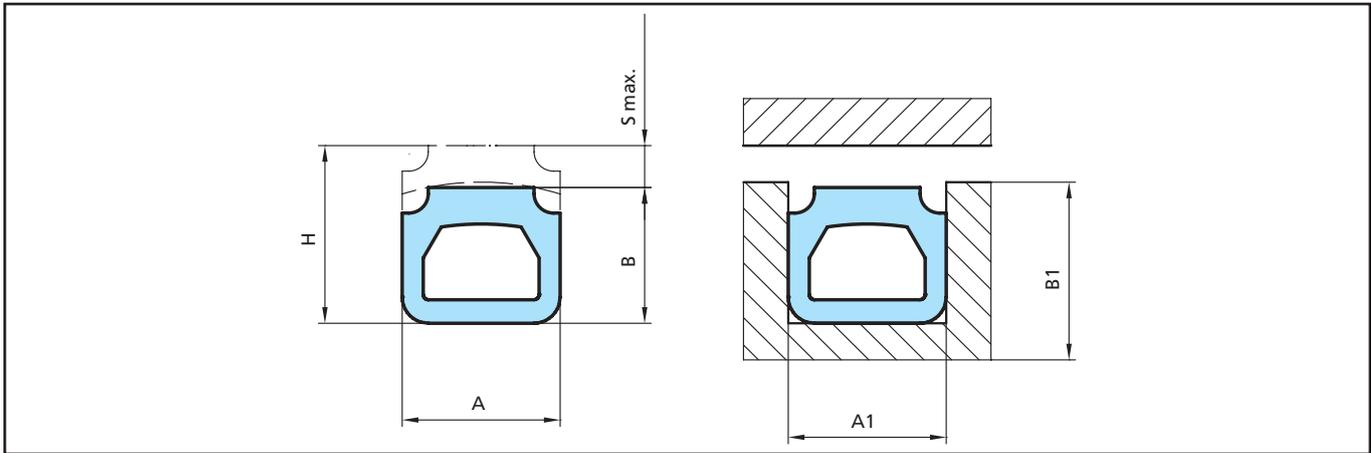
Figure 29 High-pressure profile in high purity
