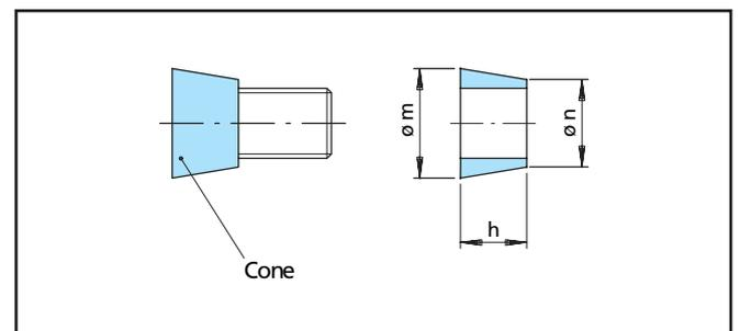
Figure 34 Cone configuration
