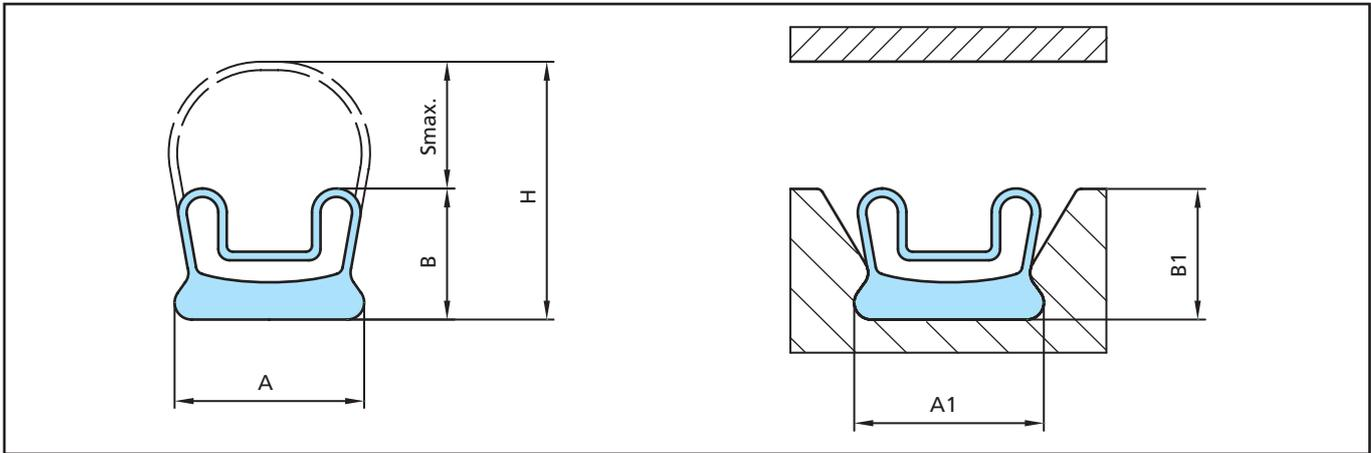
Figure 20 Low-Pressure – smooth sealing surface
