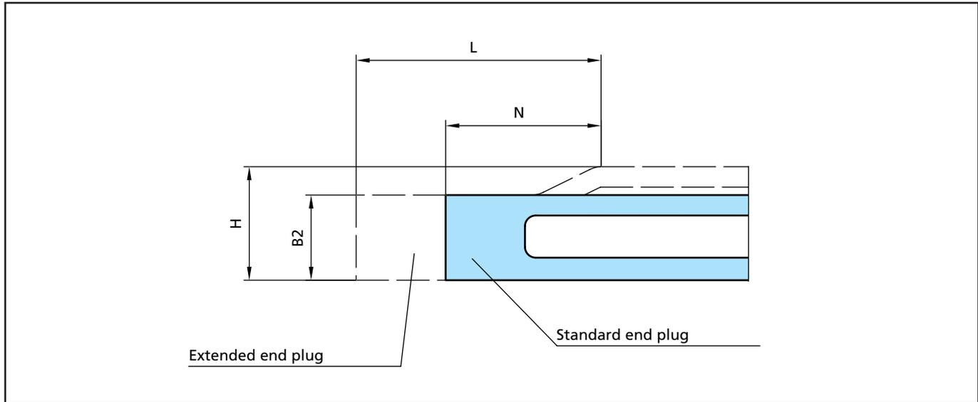
Figure 37 End plugs for high-pressure profile
