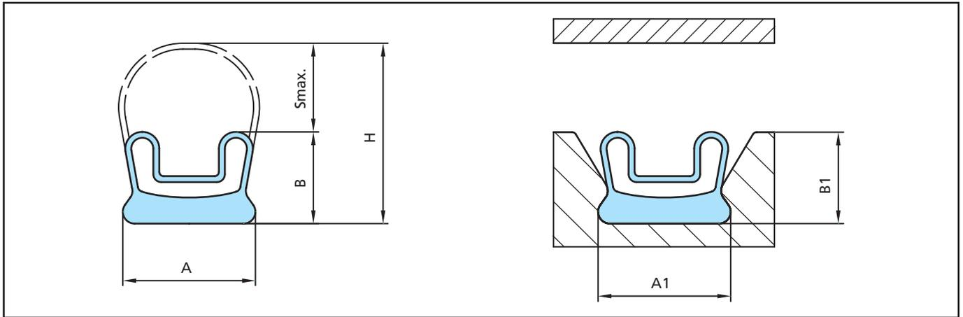
Figure 21 Low-Pressure – smooth sealing surface
