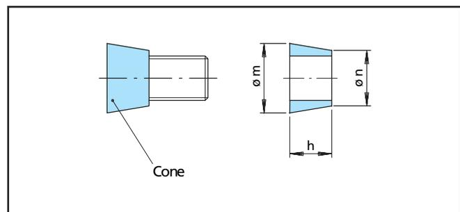
Figure 32 Cone configuration
