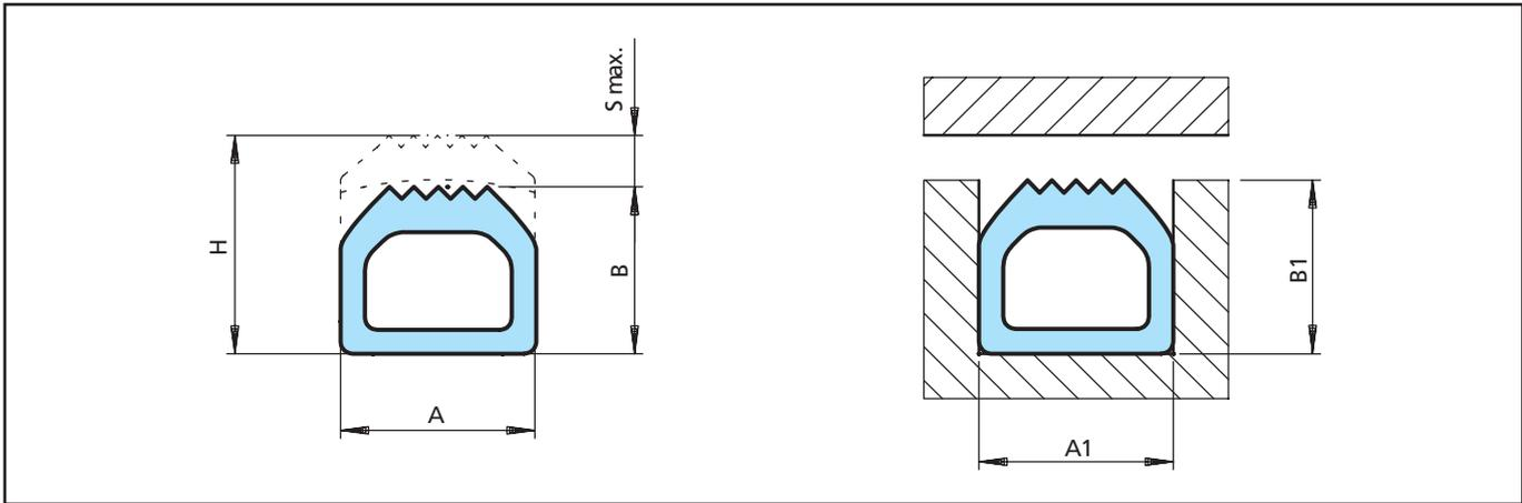
Figure 26 High-Pressure – with peaked sealing profile
