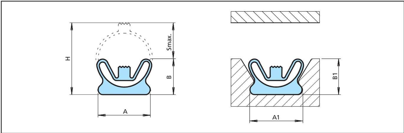
Figure 18 Low-Pressure – particularly pronounced sealing edge
