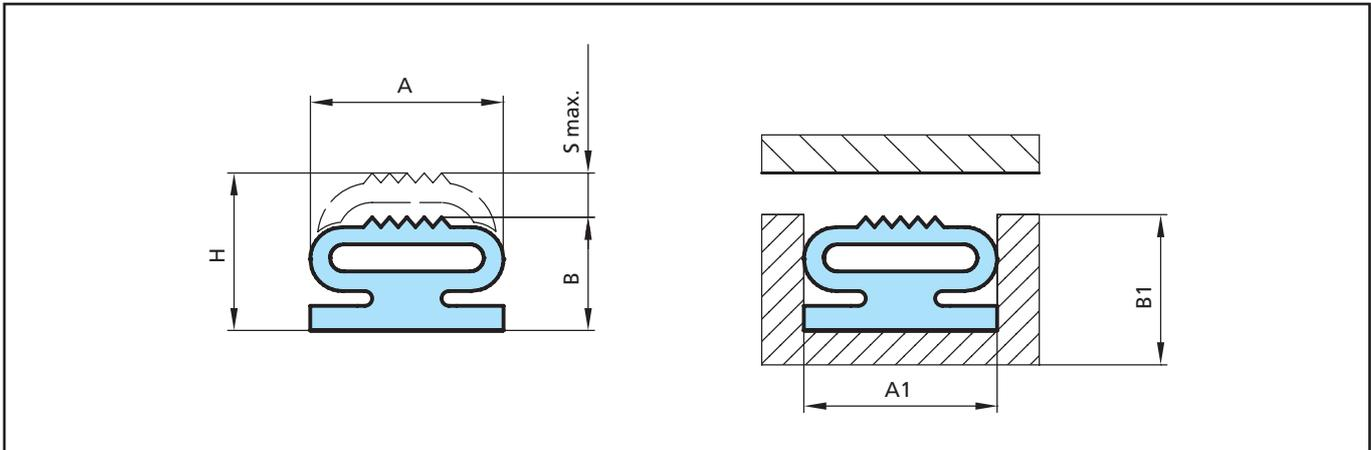
Figure 12 Low-Pressure – with peaked sealing profile
