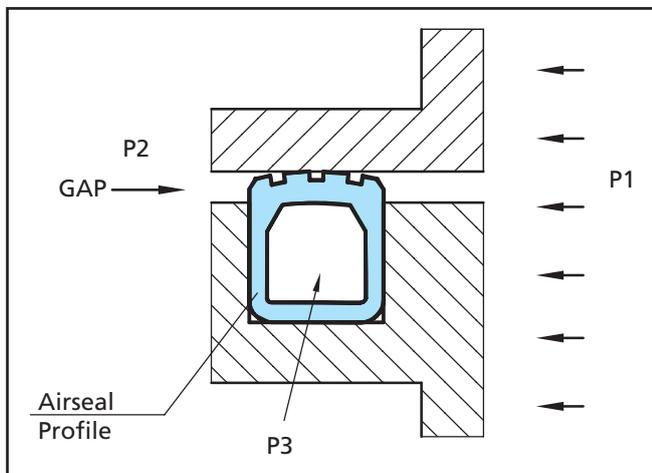
Figure 2 Pressure on Airseal
