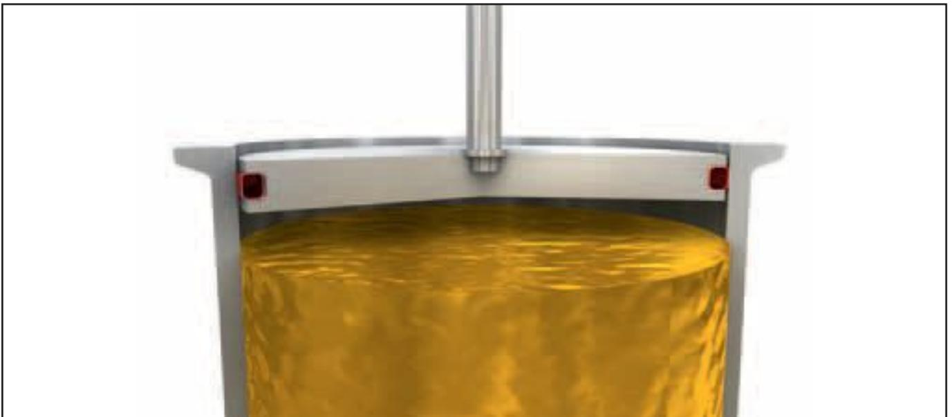
Figure 28 The Airseal expands radially outward against the inside of the drum, sealing the required gap and providing leak-tight operation under pressure.
