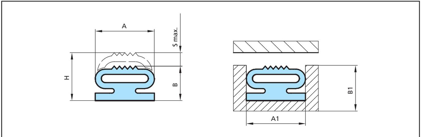
Figure 13 Low-Pressure – with peaked sealing profile
