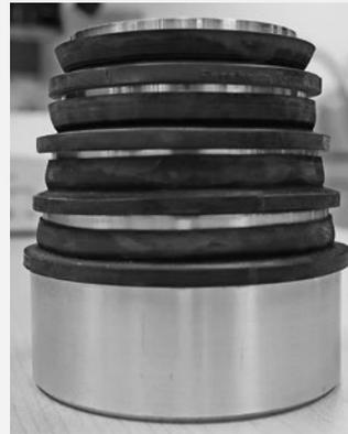
Forsheda® V-Ring in N6T50 strained at 10%, 20%, 30%, and 40% showed no cracks at any strain levels after 24 hours with ozone exposure.
