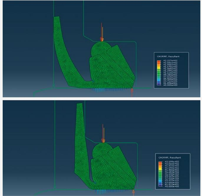
Trelleborg Sealing Solutions uses the latest practical and simulated testing approaches to predict seal behavior.
