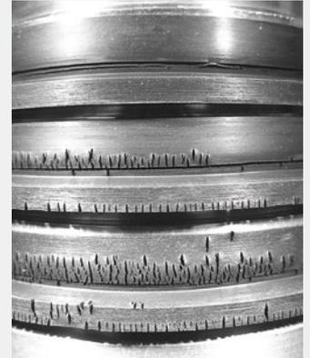
Competitor products strained at 10%, 20%, 30%, and 40% failed after 24 hours at all four strain levels with ozone exposure.
