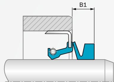
By installing Forsheda® V-Ring as shown, adequate protection is granted to the Radial Oil Seal and system service life is increased.
